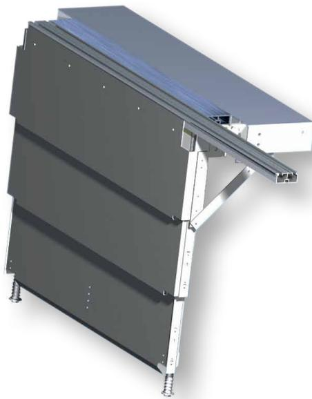
The components of the local drive are literally built into the entrance of the door frame at the lowest floor. The emergency manual lowering is positioned at the bottom of the vertical power unit.
