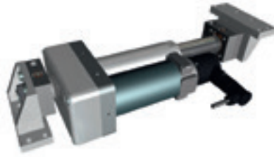
Actuator EMS 21 Up to 195 mm stroke with max. 1,680 N
