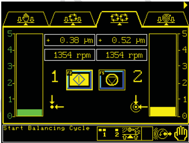
6 - Dynamic balancing for twin grinding wheel applications
