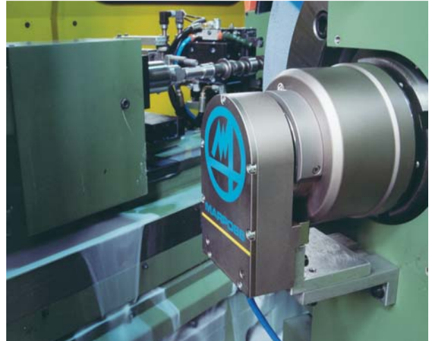
9 - External balancing head with infrared transmission
