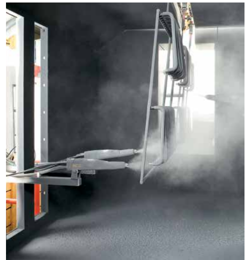
Automated powder coating
