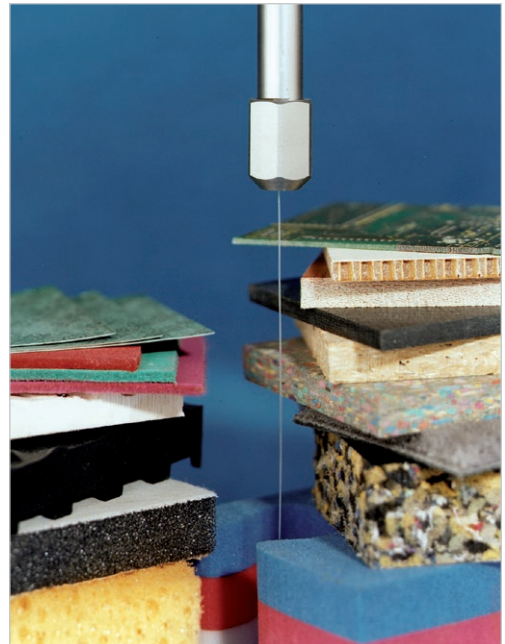
Various materials, cut with a pure waterjet.
