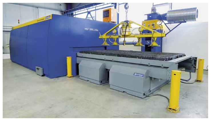
SF machine is a powerful laser cutting system for cutting of materials with a fiber laser, or a combination of fiber laser and plasma. The machine is designed for production of highly accurate parts at high cutting speeds, with surprisingly low maintenance and operational costs. The outstanding dynamics of MSF is achieved by a low-seated gantry, digital AC drives and precise planetary gears. The machine is equipped with an automatic shuttle table as standard.
