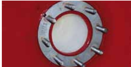
Flange for transmitter on PU pig
