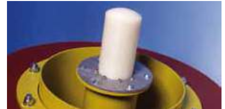
Transmitter on Flexi pig
