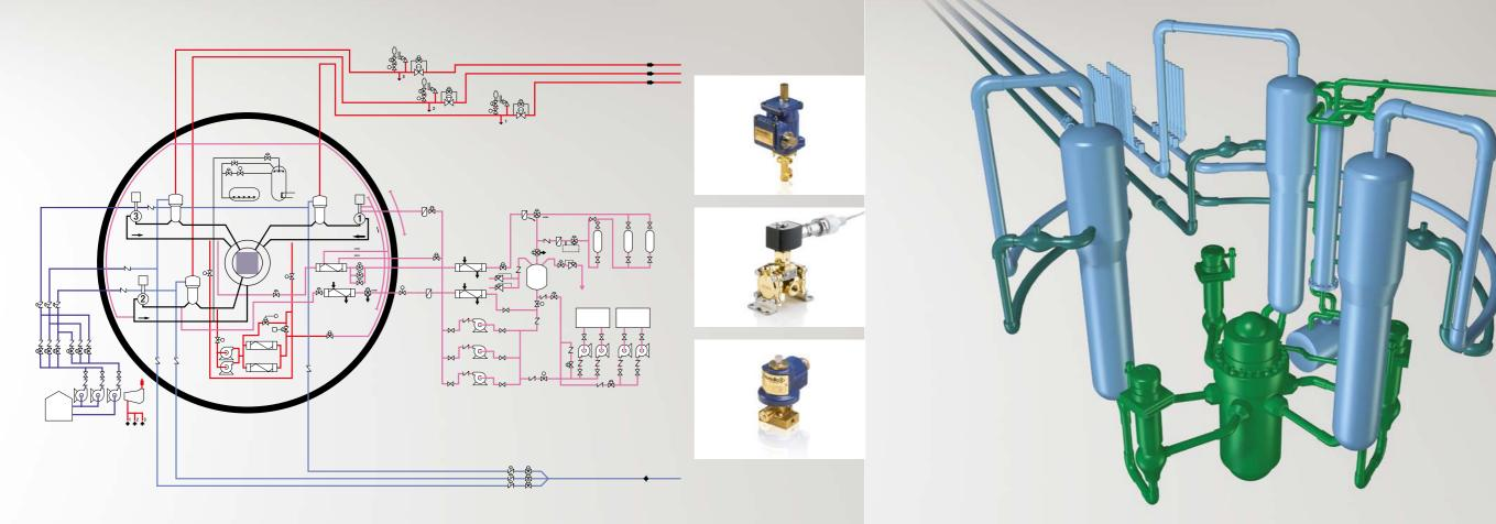
In boiling water reactor (BWR) plants, ASCO provides and supports the original equipment safety system scram solenoid pilot valves (SSPV) for hydraulic control units (HCU), and directional control valves (DCV) for control rod drives (CRD).
