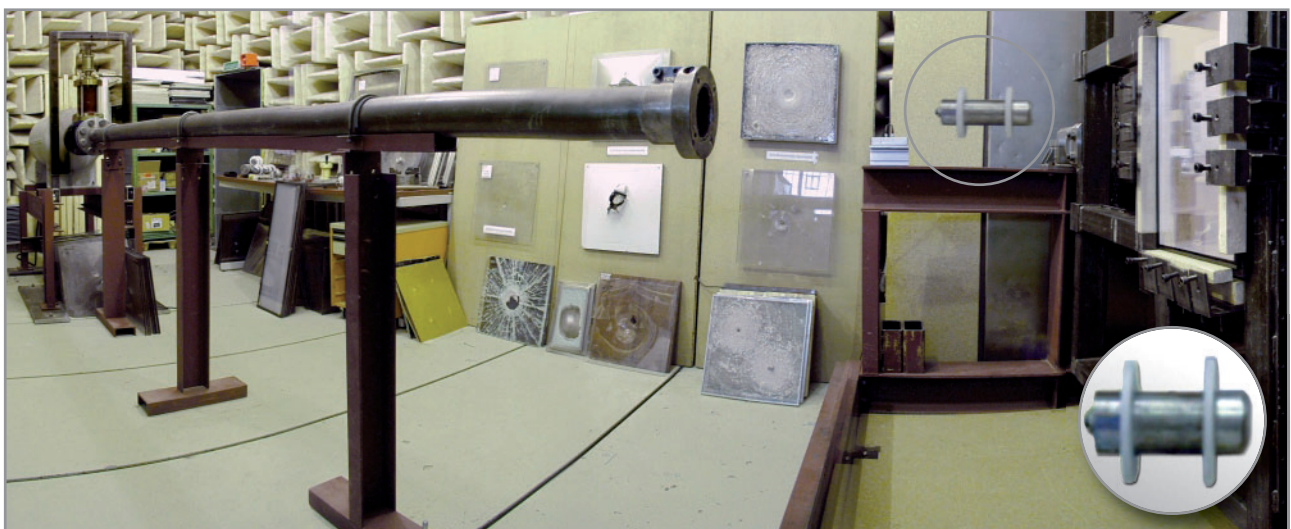
Panorama view of test laboratory at the IWF of TU Berlin. In the foreground acceleration pipe with projectile (enlarged).
