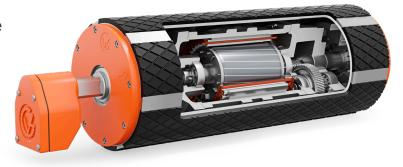
In order to achieve any heat transfer from the drum motor to the belt, the drum motor could not be covered with rubber lagging. However, most of the drum motors sold today are lagged with rubber, making it extremely difficult, if not impossible, to remove heat from the drum motor.
