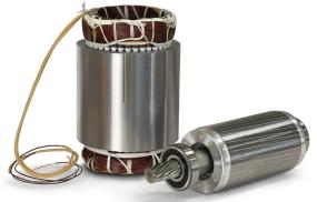
When an electric motor is running, the magnetic density produces the rotating electromagnetic field from the stator core and the rotor generates heat that needs to be dissipated. The other heat source of an electric motor is the heat generated by the copper motor windings as electricity passes through them and draws electrical current measured in ambers to produce the rotating magnetic field.
