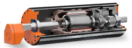
The input power cable passes through the hollow shaft and is connected to the motor stator. The electric motor is mechanically connected in-line to the gear reducer. The drum motor is partially filled with oil. The oil inside the drum motor lubricates all mechanical components and helps to dissipate heat generated by the electric motor and gear reducer onto the drum, and from the drum to the belt. In theory, the drum motor is cooled by the belt making full contact with the rotating steel drum.
