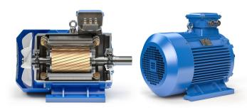
In order for an electric motor to produce rotation, a rotating electromagnetic field is needed. To achieve that, it requires ferrous and nonferrous materials, such as iron and copper or iron and aluminum. The stationary part of an electric motor (the stator) has motor windings that are copper and a laminated stator core that is iron. The rotating part (the rotor) of the electric motor is made up of iron laminations and aluminum bars.
