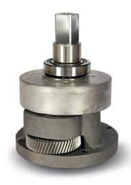
higher drum motor, an external oil cooler is required to maintain low motor and oil temperature. VDG has developed and patented a Cooling/Conditioning Unit that extracts the oil from the drum, filters it, cools it, and returns it to the drum motor. A 75 hp drum motor and higher, regardless of the manufacturer, will fail without an external oil cooler.
