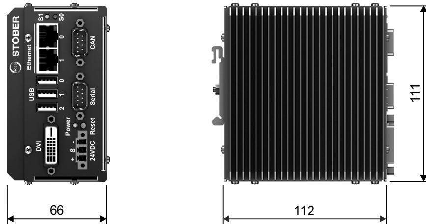
Fig. 1: Dimensions MC6x00 and MC6x01
