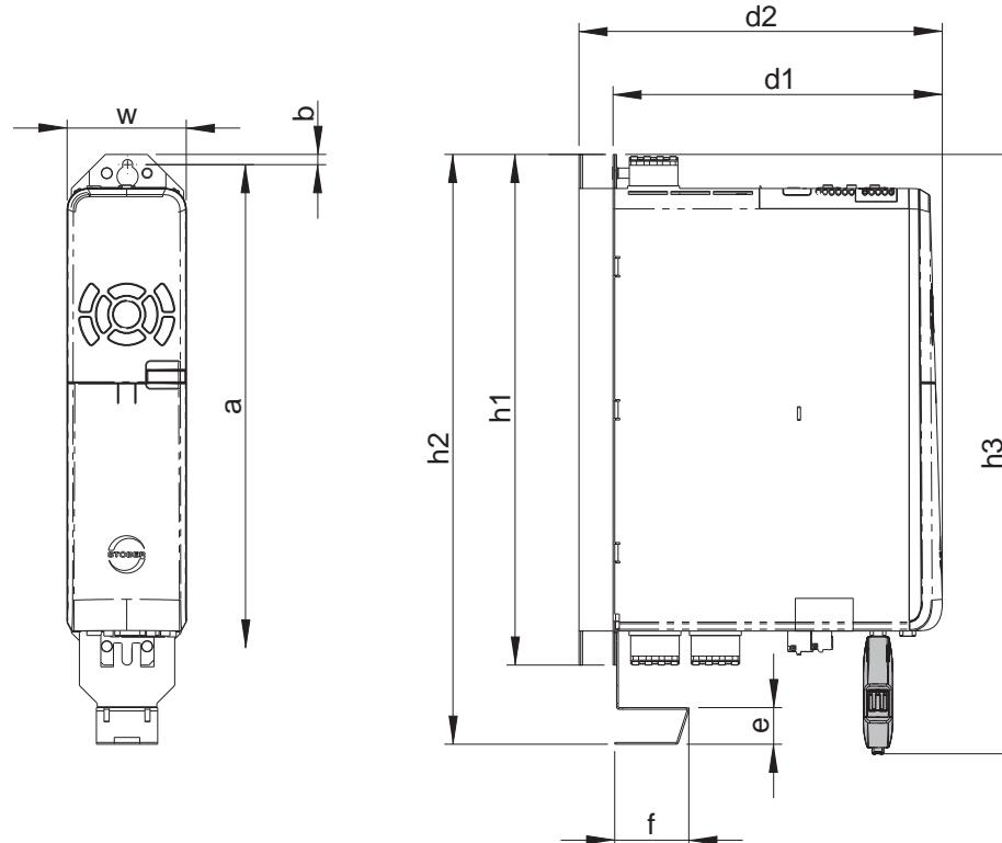
Fig. 2: SD6 dimension drawing, size 0 to 2
