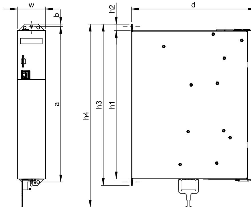
Fig. 5: SI6 dimensional drawing
