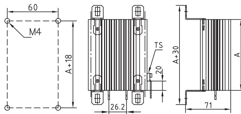
Fig. 8: Dimensional drawing KWADQU 420x91
