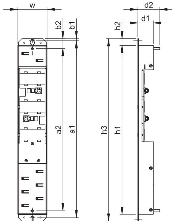
Fig. 6: DL6B dimensional drawing
