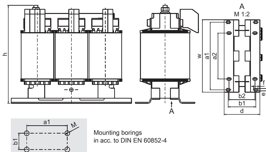
Fig. 14: Dimensional drawing TEP
