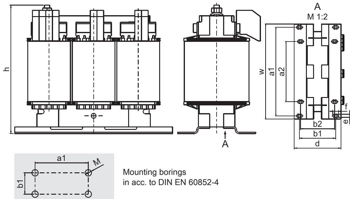
Fig. 11: Dimensional drawing TEP
