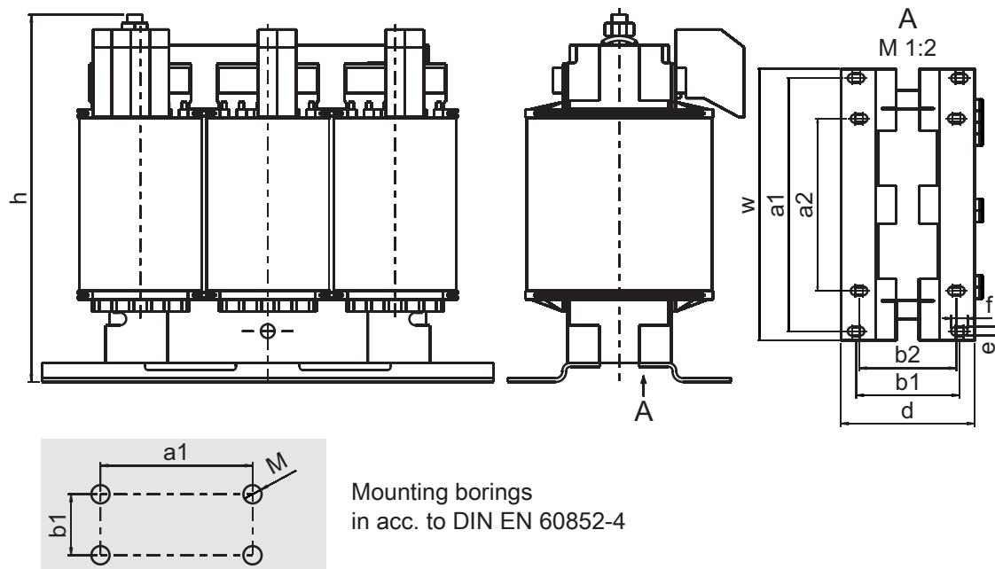
Fig. 8: Dimensional drawing TEP
