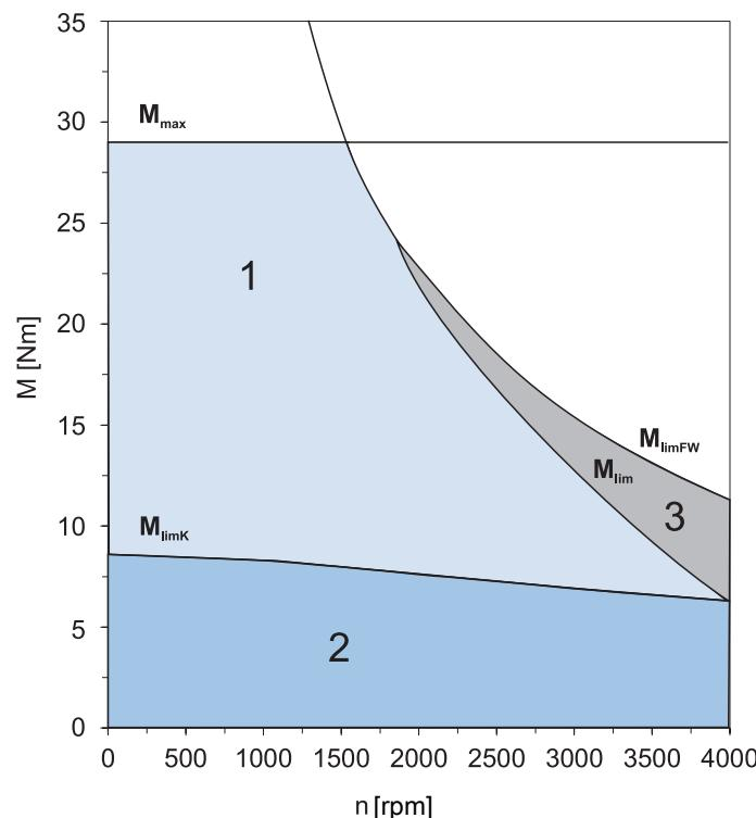
Fig. 1: Explanation of a torque/speed characteristic curve
