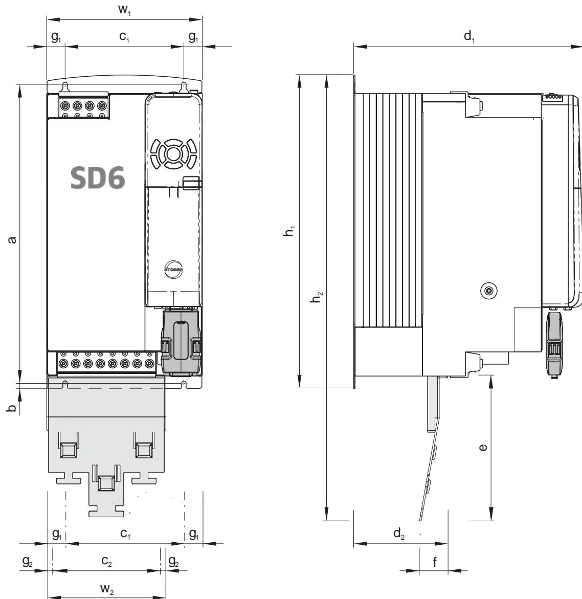
Fig. 3: Dimension drawing SD6, size 3
