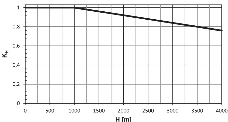
Fig. 4: Derating depending on the installation height
