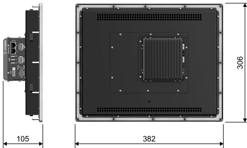
Fig. 2: Dimensions MC6x10 and MC6x11
