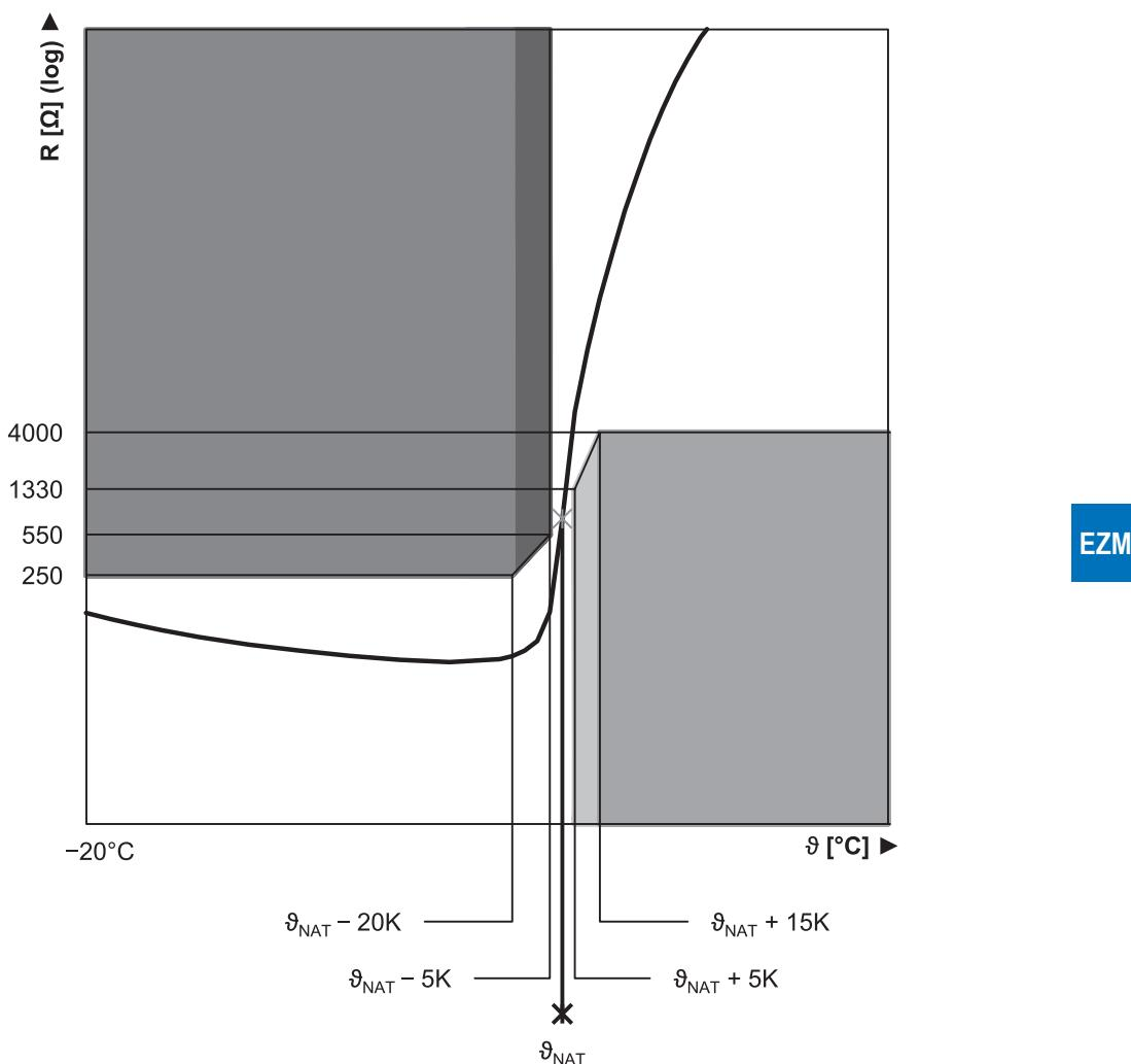
Fig. 2: Characteristic curve of PTC thermistor (single thermistor)
