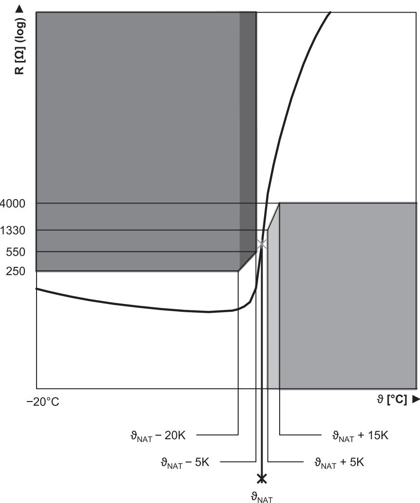
Fig. 2: Characteristic curve of PTC thermistor (single thermistor)
