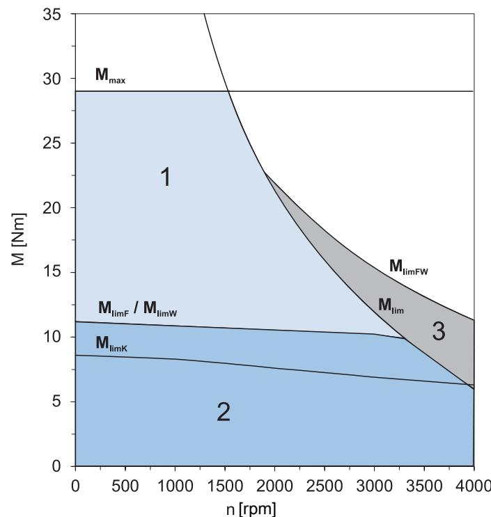
Fig. 1: Explanation of a torque/speed characteristic curve
