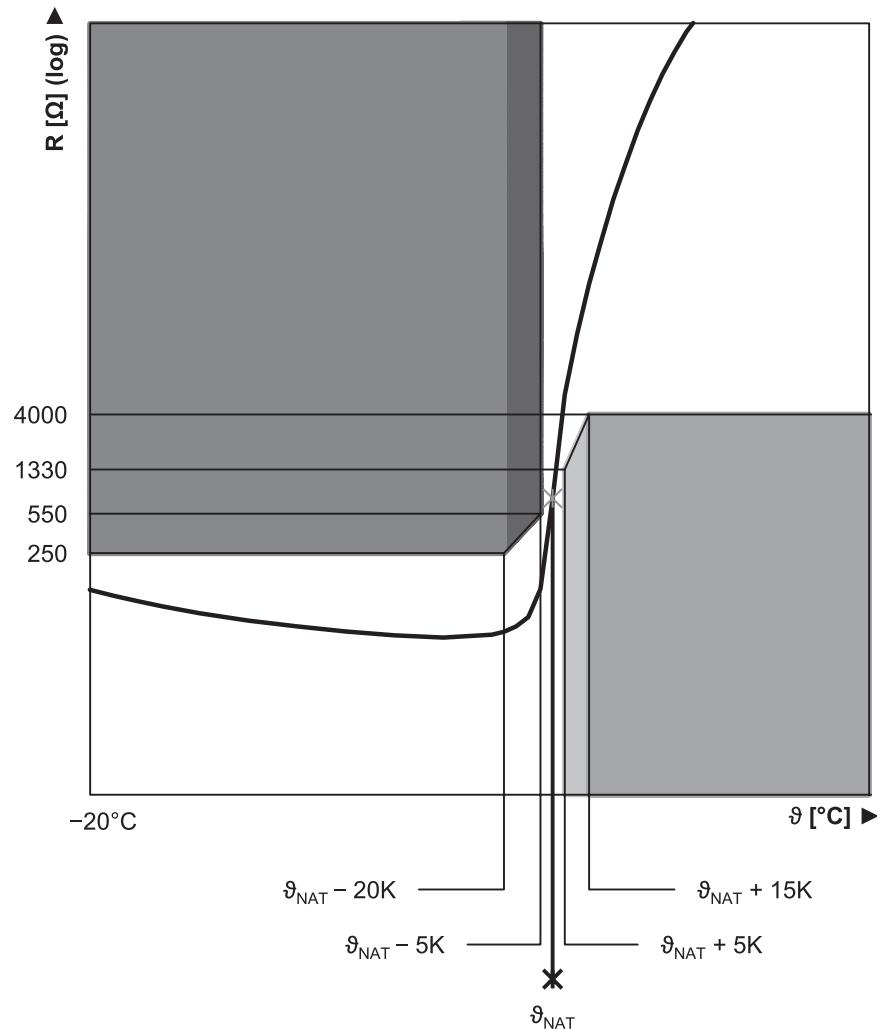
Fig. 2: Characteristic curve of PTC thermistor (single thermistor)
