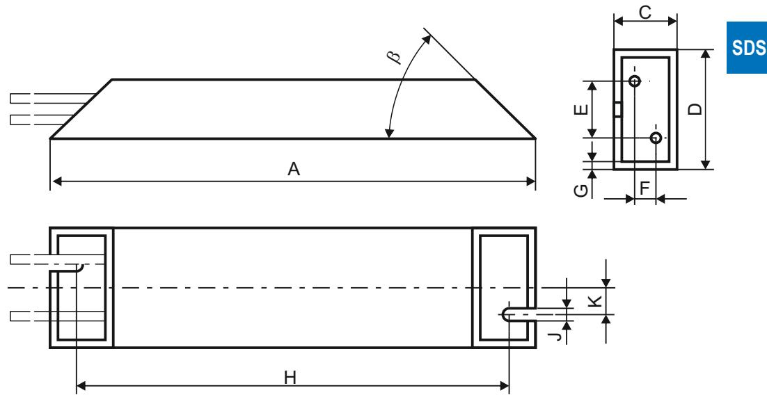
Fig. 3: Dimensional drawing GVADU, GBADU
