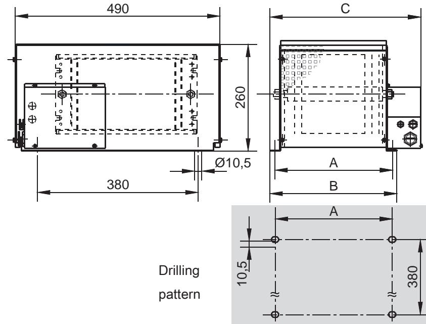
Fig. 4: Dimensional drawing FGFKU
