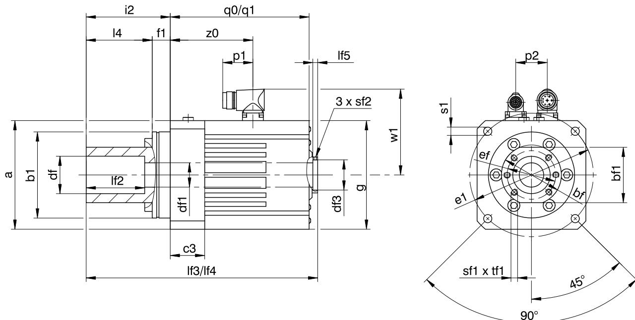
q0, lf3 Applies to motors without holding brake. q1, lf4 Applies to motors with holding brake.
