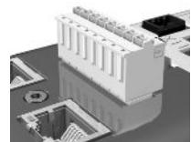
The ST6 accessory makes it possible to use the "Safe Torque Off" (STO) safety function in the SD6 drive controller in safety-relevant applications according to EN ISO 13849-1.
