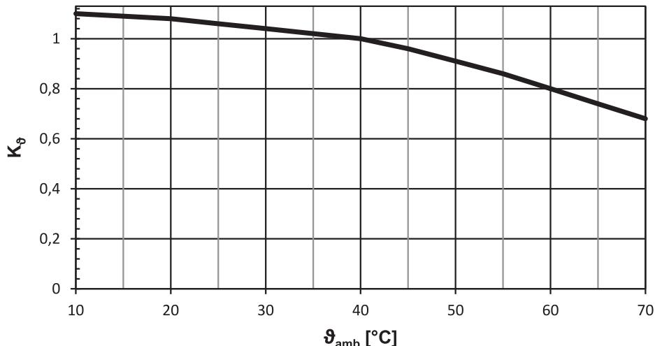
Fig. 3: Derating depending on the surrounding temperature
