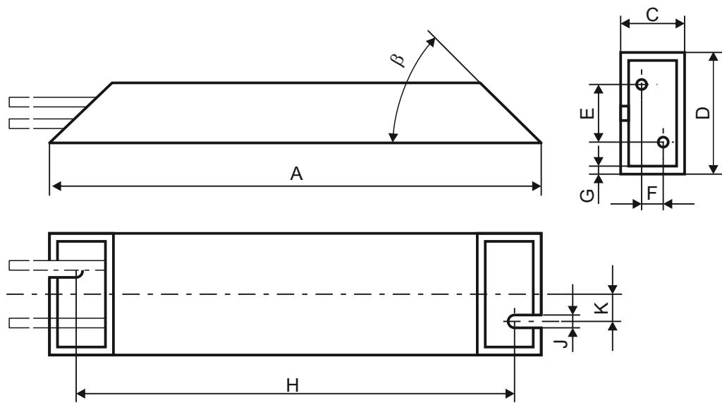
Fig. 5: Dimensional drawing GVADU, GBADU
