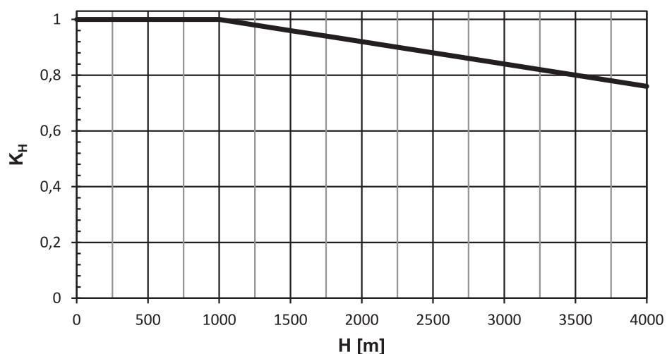
Fig. 4: Derating depending on the installation height
