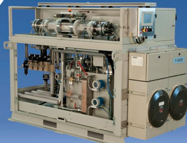
**PEROXIDE DOSING PUMPS** with intensifier in "single" and "stand-by" design, pressure range up to 350 MPa, flow rates up to 150 l/h, as well as high pressure tubing systems and injection nozzles for use in LDPE (Low Density Polyethylene) reactors.
