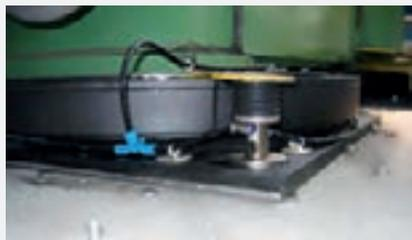
Very robust galvanised proportional valve. Level accuracy is approximately  $\pm 1/10$  mm. Suitable for Bilz FAEBI®, FAEBI®-HD and BiAir® air spring insulators.
