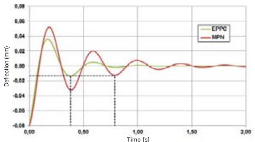
Theoretical MPN vibration curve compared with EPPC™. At a deflection of  $-80 \mu\text{m}$  the MPN reaches a stable position within a tolerance of  $\pm 15 \mu\text{m}$  after 0.75 seconds. With EPPC™ the deflection time is reduced by 45 % to 0.4 seconds.
