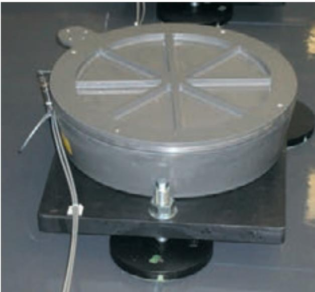
The foundation insulation using low-frequency BiAir® membrane air springs enables an optimum insulation effect.
