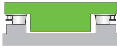
Vibration insulation concrete block or steel platform
