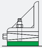
Stable connection to the machine bed using **bolt-on installation fittings** that remain in place when the machine is lifted. Specifically for machines with high dynamic forces (injection moulding machines, stamping equipment, etc.).
