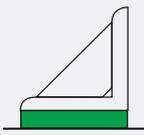
**Free-standing** machine foundations using Bilz insulation pads with low demands on alignment. The uneven floor is compensated for with pads, etc. The arrangement of the pads is usually a pattern of points, not over the full surface. Number and size of the required insulation pads is given by the weight of the machine and the existing support surface.
