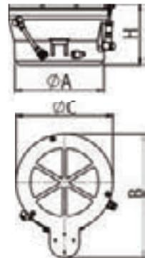
\* For the sizes 1 to 3 of series ED/HE-MAX the ØA is the same as ØC (piston diameter)
