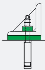
**Bolt-through** ground anchoring using insulation pads and insulation washers. The use of insulation washers prevents vibrations being transmitted through the bolt.
