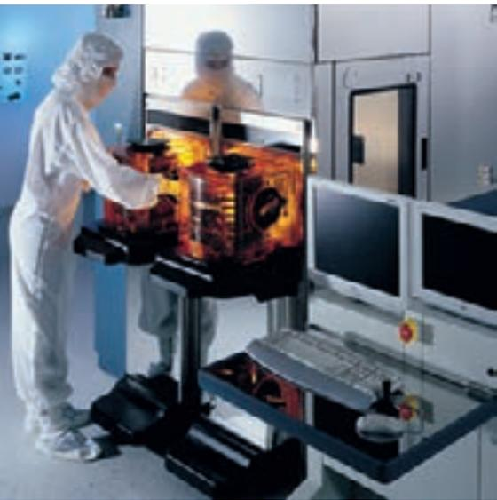
COMPASS PRO Wafer Inspection Machine
