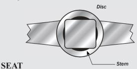
The MK Butterfly Valve seat is constructed by bonding a resilient elastomer to a rigid back-up ring, which forms the outside periphery of the seat. Slip fitted in the valve body, the seat is **field replaceable** without special tools. In the closed position, the disc rim and stem seal lands form an uninterrupted line of sealing contact with the resilient seat, to assure **drop tight sealing** at rated shutoff pressure. MKP seats is offered in a wide range of materials.
