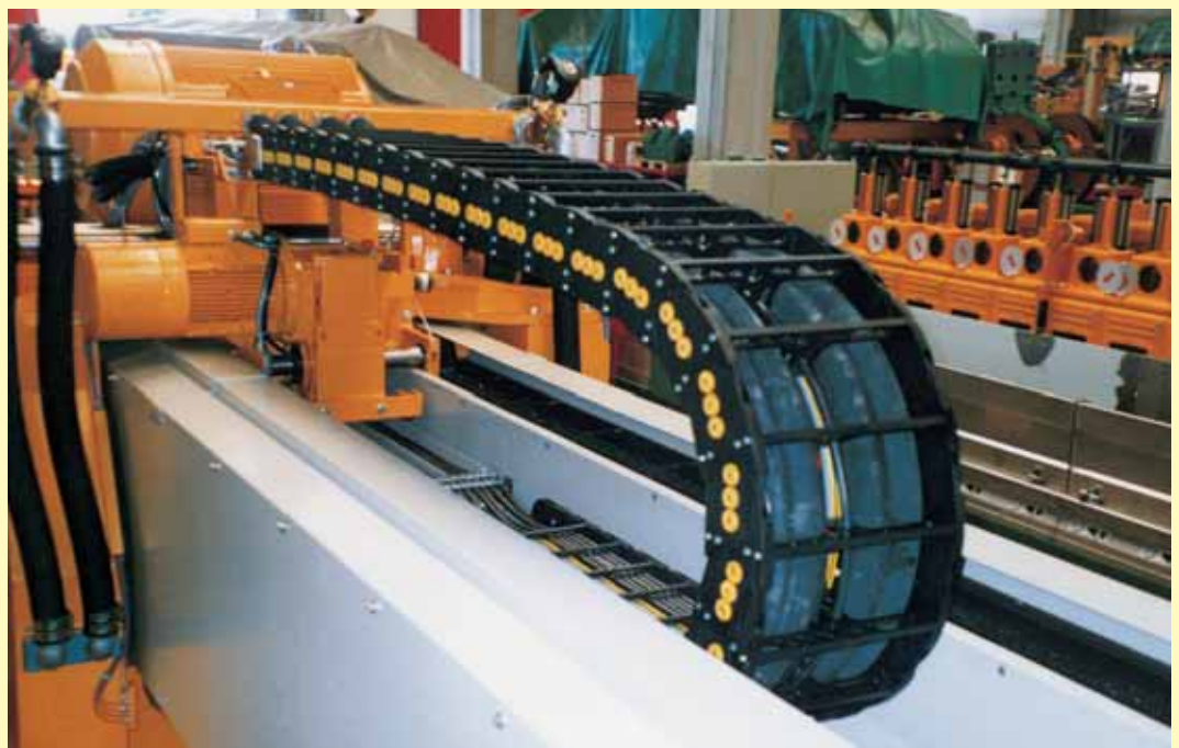
Nylon chain, type 310, in a self-supporting state.
