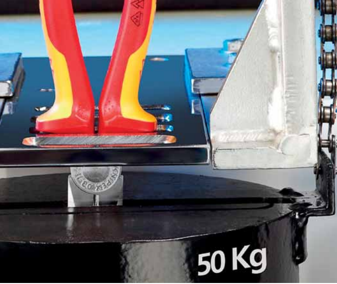
Testing the adhesion of the insulating coating at 500 N.
