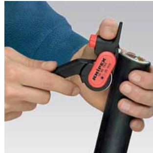
Setting the tool for longitudinal cut
