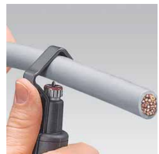
Setting the tool for circular cutting
