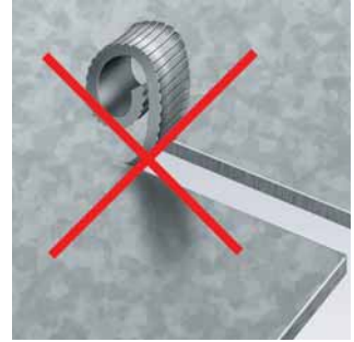
Notching without chip breaking
