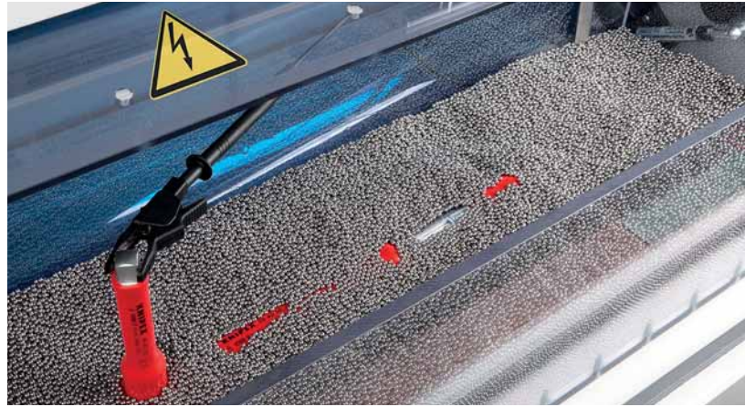
Testing the electrical insulating properties.
