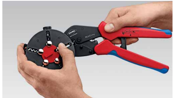
Changing the crimping dies: unlock the magazine position, take out the set of dies which the pliers have been pushed on
