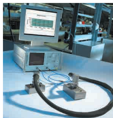
MICROSTRIP INJECTION TEST BENCH TO CONTROL TRANSFER IMPEDANCE
