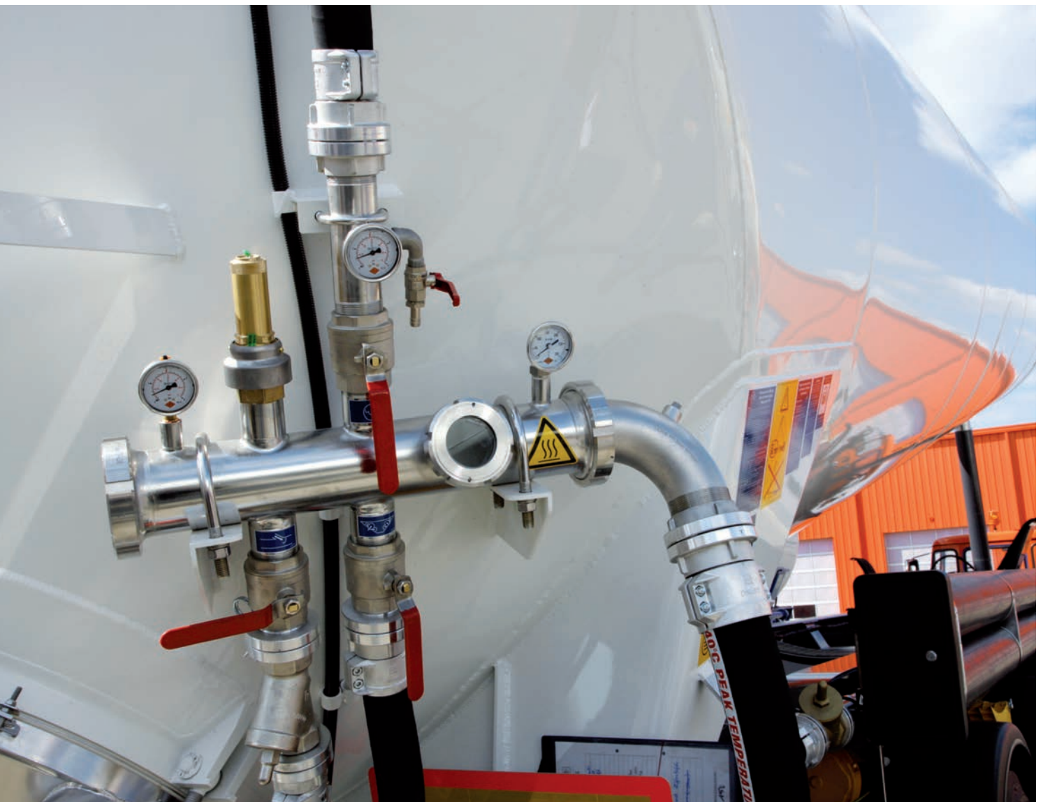
Open discharge safety valve installed on a silo trailer application
