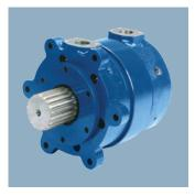
MV125 - 300 rpm 6903 lb-ft (9359 Nm) Offered in A [3000 psi (207 bar)] or H version [4500 psi (310 bar)]. Splined, tapered, straight keyed, female, and double output shafts are standard, along with through holes to 3". Optional thrust and radial load bearings with substantial capacity, tach pickups, double stacks, and brake mounts available.
