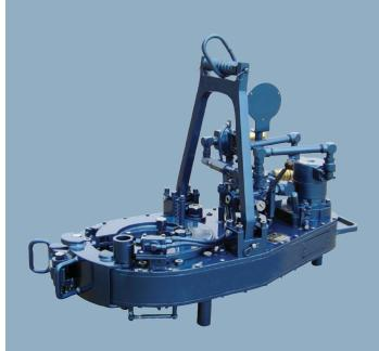
Caisson drill rigs use 4-ported motors along with a multispeed circuit to vary bit rpm and torque. ▲ Power tongs are a staple of the oil field. Our vane crossing vane motors have been providing the torque to make and break pipe joints for over 40 years.
