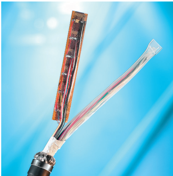
Picocoax ® wires soldered onto a PCB
