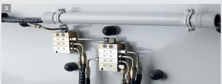
The automatic central lubrication system guarantees a maintenance-free lubrication of all bearings and seals.
