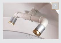
7 | Production water is sprayed into the mixer through multiple nozzles.
