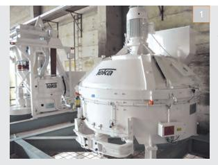
1 The THT mixer is ideally suited for face-mix, fiber-, foam-, self-compacting-, color-, ultra-high-strength concrete, etc. This mixer type is also optimally suited for the absolute smallest batch sizes (partial loadings), and therefore extremely variable in its use.
