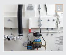
5 THT mixers have low maintenance factors. and require gearbox oil changes only every 2,500 hours. Central grease lubrication (except for rotating mixing stars) is standard. An optional motor-driven automatic grease lubrication pump is available.
