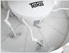
1 The mixer pan floor and walls are protected by replaceable wear liners. Depending on the application, wear liners are made of either A.R. steel, chillcast tiles, hard faced steel, or ceramic tiles.
