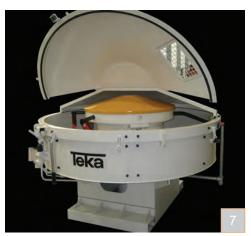
**7** A protective mixer hood encloses the mixer pan. A built-in seal makes it near dustproof. Large, hinged segments with variable openings are possible, raised and lowered by a manual- or motorized cable winch. With no components located above the mixer hood, there are no obstructions to impede the arrangement of cleaning segments,
