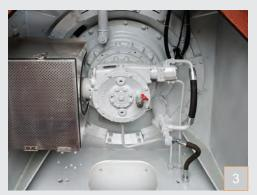
3 The centrally located planetary gearbox is driven by a 3-phase TEFC motor which is flangemounted directly to the gearbox, in the case of mixer sizes THZ 375 to THZ 750.
