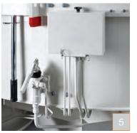
**5** | The discharge gate assembly, used to remove the batch from the mixer, is a complete heavy-duty component bolted to the mixer pan floor. The semi-circular gate is hydraulically operated by means of a rotary cylinder. It is electrically controlled and can be opened to any degree desired. Locating the pivot-point of the gate slightly inside the pan circumference allows for a large opening and thereby, a fast discharge. In case of a power outage,
