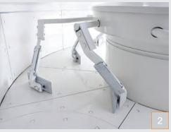
2 Central lubrication for the mixing arm bushings is available. Depending on the application, mixing paddles, wall scrapers, and mixing arm wear guards made of
