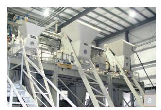
8 Depending on the plant design, charging the mixer by means of a skip hoist is possible. TEKA offers tilting skip hoists as well as the non-tilting, bottom discharge type. Inclination of the hoist track from 45° to 90° may be specified.
