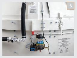
6 | TPZ mixers have low maintenance factors, and require gearbox oil changes only every 2500 hours. Central grease lubrication (except for rotating mixing stars) is standard. An optional motor-driven automatic grease lubrication pump is available.
