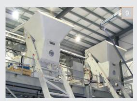
9 | All TEKA mixers can be outfitted with a Skip Hoist to charge the mixer with batch materials. **TEKA offers** tilting skip hoists for very steep angles
