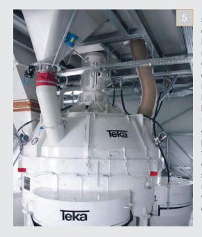
5 | The mixer hood design has several large spaces for material inlets. Cleaning/access doors can be installed in various locations, and are built with quickrelease latches, gas-pressure pistons to keep them open, and electronic safety switches to stop mixer operation when they are opened.
