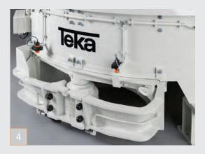
4 | Separate hydraulic power packs operate the discharge gate(s). A manual hand pump is included to open discharge gates in case of a plant power outage. Discharge gate openings are large for short discharge times, but can also be opened to various degrees using proximity switches.
