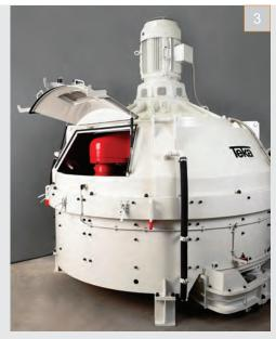
3 | The robust and compact design of the drive line uses only one motor for high efficiency. Hydraulic Turbo Couplings are standard on the TPZ 1500 and larger models. As an option, a frequency converter can be installed on all TEKA mixers, to optimally adjust the speed of the mixing arms.
