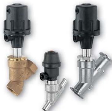
GEMÜ 554 2/2-way globe valve, metal, pneumatically operated, plastic piston actuator Control function: Normally closed (NC), Normally open (NO), Double acting (DA)
