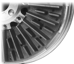
Cross-drilled rotor with heat dissipating fins.
